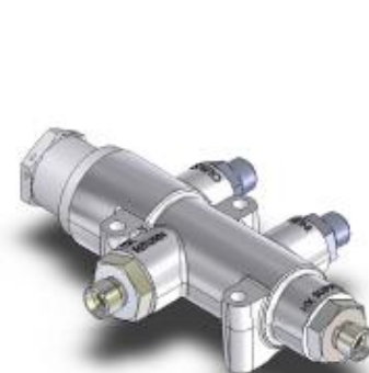
9636 HEAT EXCHANGER BYPASS VALVE A thermal and differential pressure operated valve that regulates hydraulic flow to the heat exchanger. Includes a function to bypass the heat exchanger when it is contaminated.
