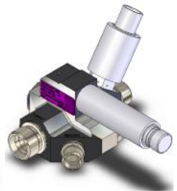
8263 BRAKE SELECT VALVE Solenoid operated valve which purfs hydraulic pressure to supply the Main Landing Gear brakes.
